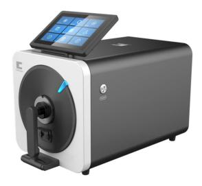
CS-822 bench-top spectrophotometer is with the 45/0 geometry. 45/0 geometry is close to the visual perception color value, which can exclude the specular light on the textured surface. It is suitable for color measurement of automotive interior parts, textiles, coil coatings, plastic products, coatings, packaging and other materials color measurement.
